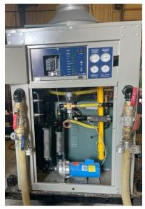
Figure 28 - Primary Circulation Line Connections
