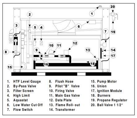
Figure 29 - Water Heater Cabinet Diagram
