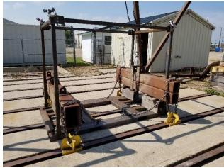
**Figure 1**. 2100-1200 system base frame and installed lifting frame assembly secured to test bed.
