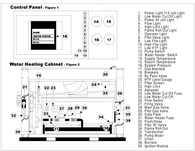
Figure 43 - Control Panel & Water Heater Cabinet Layout
