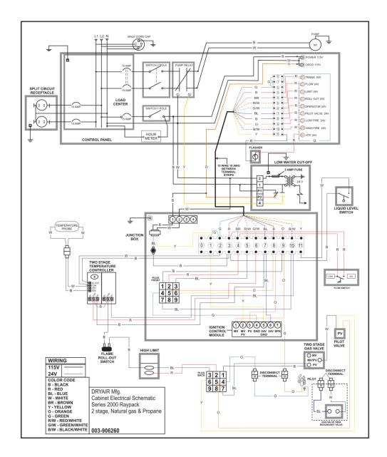
Figure 49 2000-1200 Central Heating Unit Electrical Schematic
