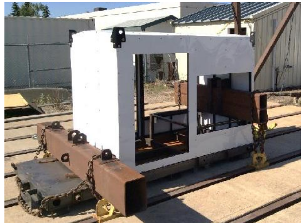
Figure 1. Bare 200GTS assembly with lifting lugs attached at the four corners.
