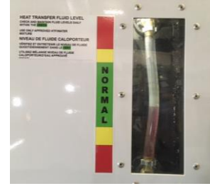
Figure 27 - HTF Level Indicator
