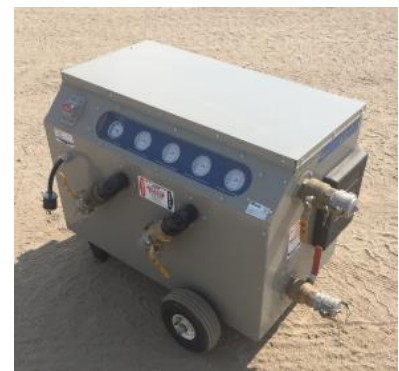
Figure 11 - Plate Heat Exchanger Unit
