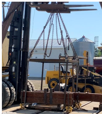
Figure 3. Test set-up for application of force to test bed.
