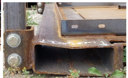
Figure 5. Deformation of the system base near the lifting frame corner post mount bracket.
