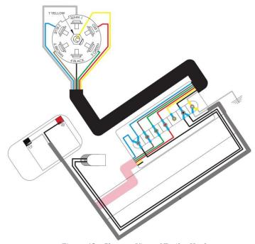
Figure 45 - Close-up View of Trailer Hook-up
