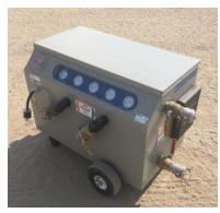
Figure 10 - Plate Heat Exchanger Unit
