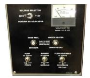
Figure 27 - Control Panel Pump Switch
