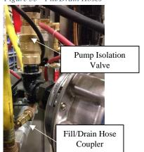
Figure 34 - Pump Connections
