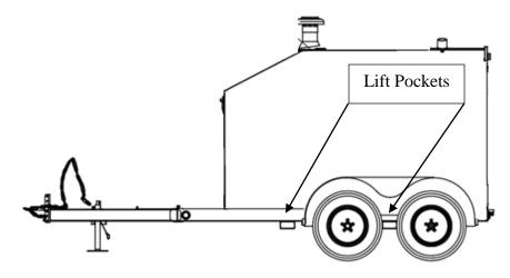
Figure 14 - Lifting Points
