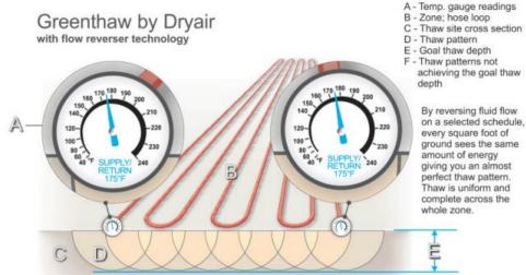
Figure 12 - Flow Reverser Technology, Even Thaw Pattern
