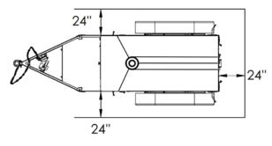
Figure 16 - Top-View Clearances
