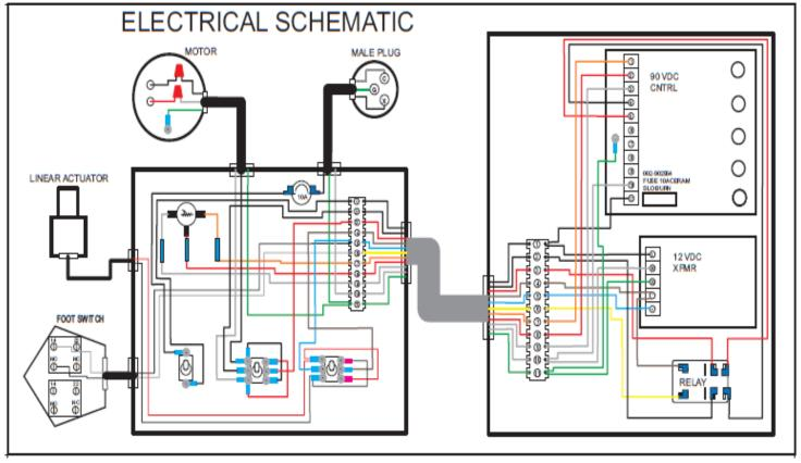
Figure 44 - 400 GTS Hose Reel Electrical Schematic
