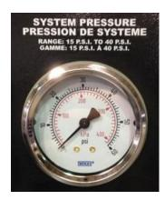
Figure 25 - System Pressure Gauge
