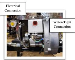
Figure 22 - Riello Burner, Cover Removed
