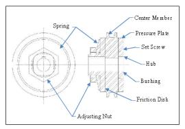
Figure 40 - Torque-limiter clutch
