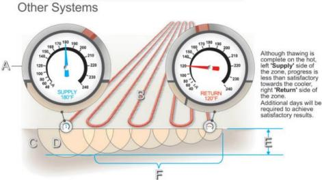
Figure 13 - Without Flow Reverser Technology, Uneven Thaw Pattern
