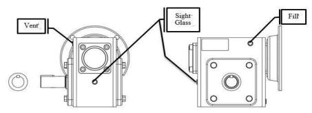
Figure 39 - Oil Fill Location Gear Box
