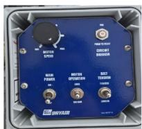
Figure 36 - Hose Reel Control Panel
