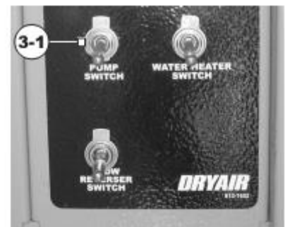
Figure 17-Pump, Water & Flow Reverser Switch
