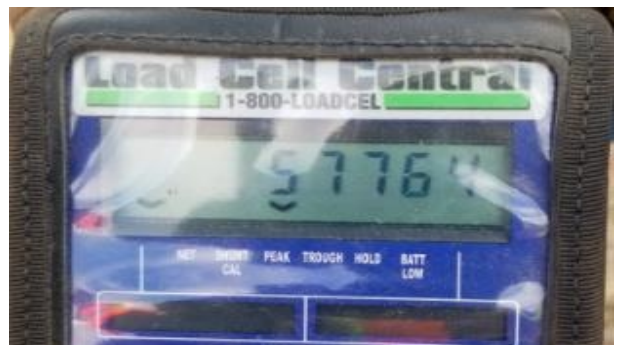
Figure 4. Peak force applied during the lifting frame test.
