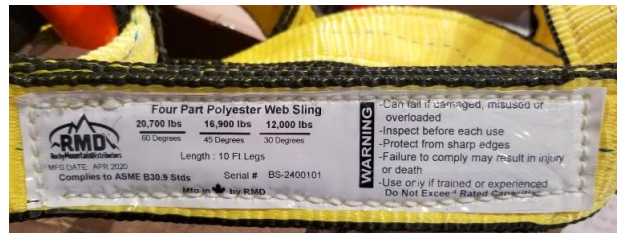
Figure 2. Polyester web sling intended to be used to lift 650GTS at four corner post lifting bracket locations.
