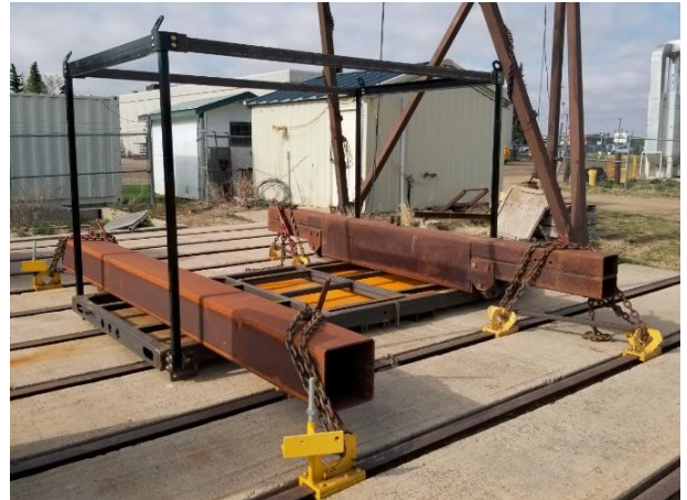
Figure 1. 650GTS trailer frame and installed lifting frame assembly secured to test bed.
