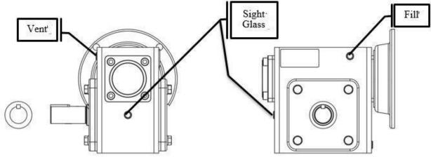
Figure 46 - Oil Fill Location Gear Box
