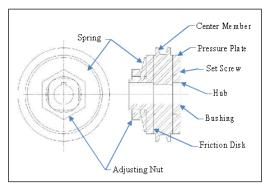
Figure 47 - Torque Limiter Clutch
