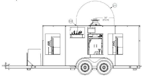
Figure 14 - Top-View Clearance
