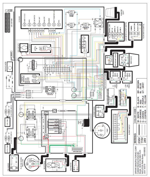
Figure 51 - 900 GTS Flex Electrical Schematic
