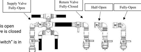
Figure 30 - Supply and Return Valve Positions
