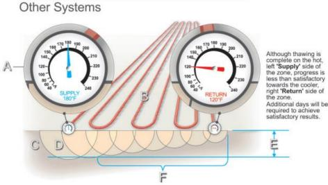
Figure 13 - Without Flow Reverser Technology, Uneven Thaw Pattern
