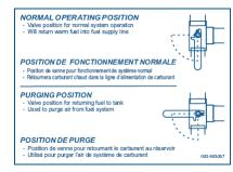
Figure 31 - Fuel Line Valve Positions
