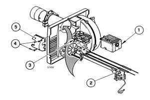
Figure 34 - Removing Burner Drawer Assembly
