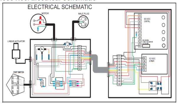
Figure 52 - Hose Reel Electrical Schematic
