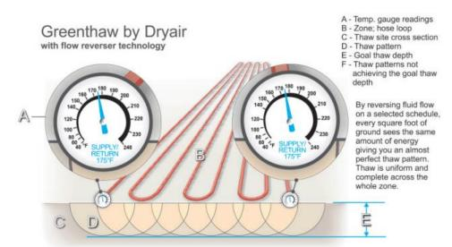
Figure 12 - Flow Reverser Technology, Even Thaw Pattern
