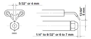
Figure 36 - Ignition Electrode Setting
