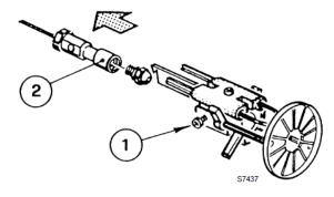
Figure 35 - Burner Nozzle
