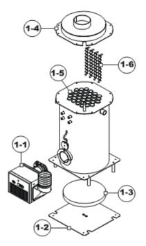
Figure 48 - Heat Exchanger Breakdown
