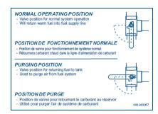
Figure 29 - Fuel Line Valve Positions
