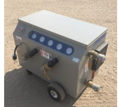
Figure 9 - Plate Heat Exchanger Unit
