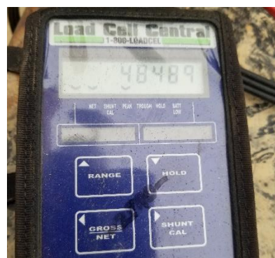
Figure 4. Peak force applied during the lifting frame test.
