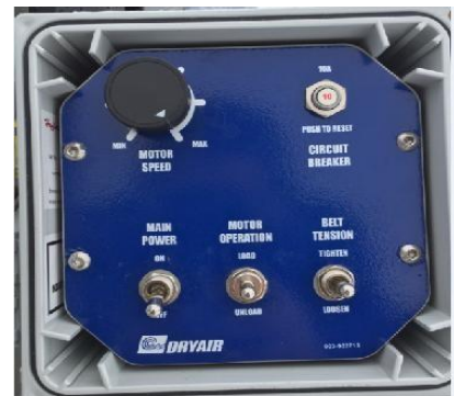
Figure 37 - Hose Reel Control Panel
