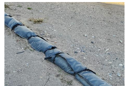
Figure 9 - Insulated Line Jackets
