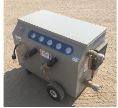
Figure 6 - Plate Heat Exchanger Unit
