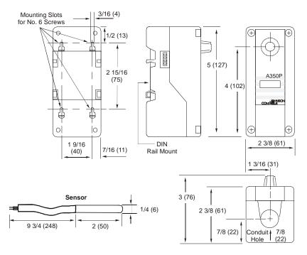
Figure 6: A350P Control and Sensor Dimensions, in. (mm)
