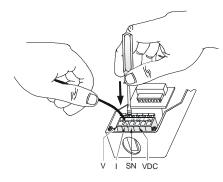
Figure 7: Cage Clamp Terminal Block
