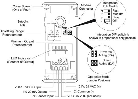
Figure 2: Interior View Showing A350P Control's Features
