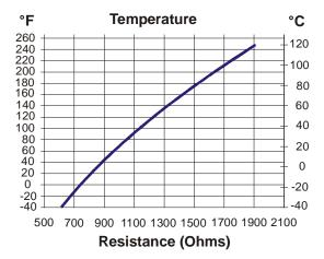
Figure 8: Temperature vs. Resistance Chart for the A99B Series Sensor
