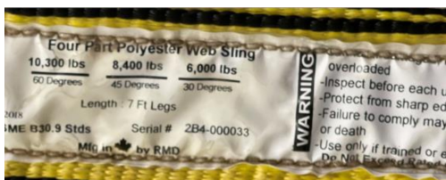
Figure 2. Polyester web sling intended to be used to lift the 2100-0900 at four corner post lifting bracket locations.
