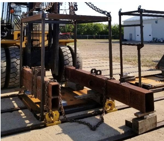
Figure 1. 2100-0900 system base frame and installed lifting frame assembly secured to test bed.
