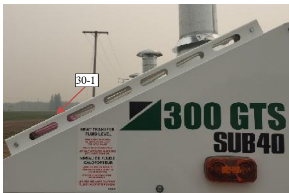
31-Glycol level sight gauge
