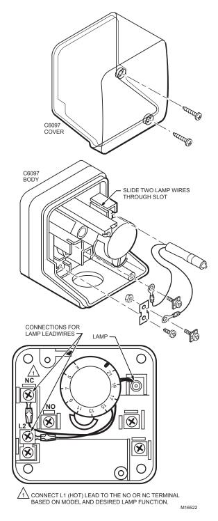
Fig. 4. Installing the Position Indicator Lamp Kit.
