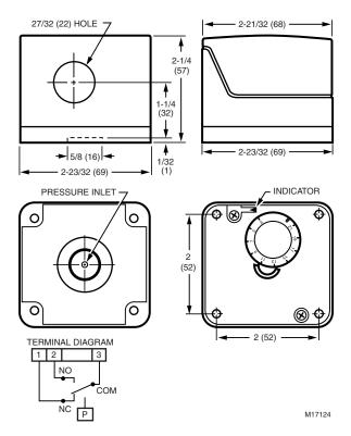
Fig. 2. C6097 Flange Mount dimensions in in. (mm).
