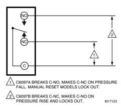
Fig. 9. C6097 schematic.
