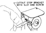
Fig. 5 -- All models have a screw type cutout stop. The stop screw must be loosened and moved to the stop setting desired. Tighten screw after setting is made.
