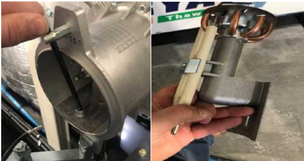
Removing the Turbulator
