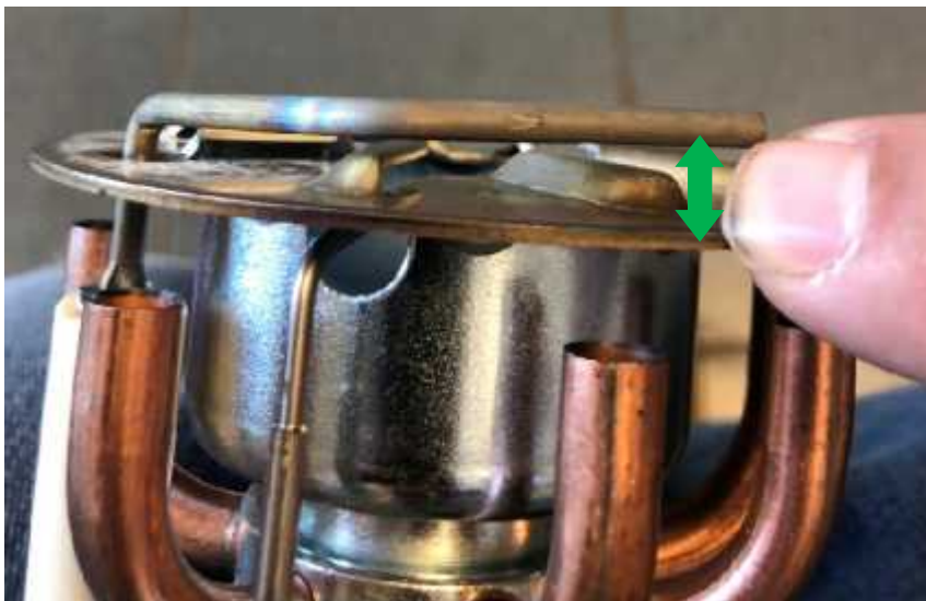
Spacing between probe and plate 3/16"
