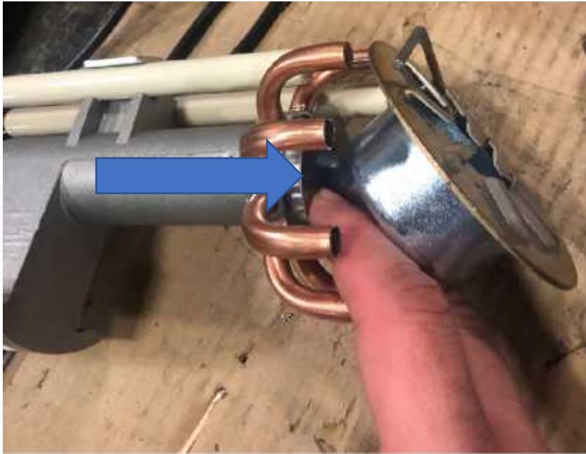
Insert Spacer Washer (propane orifice)
