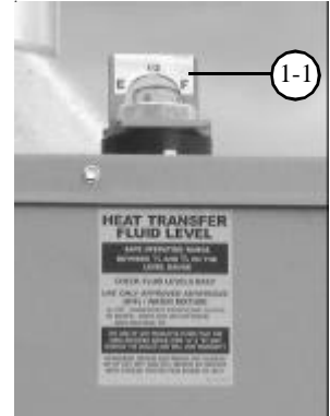
1 - HTF level gauge
