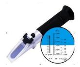
Figure 3-1 Refractometer
