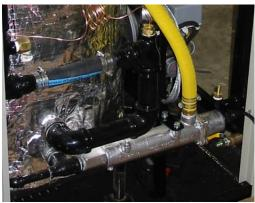
Figure 5-6 Cold Start Fluid Pre-Heater
