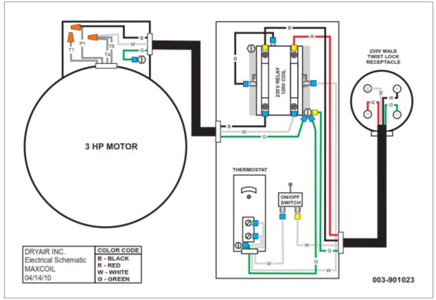
Figure 8-6 Model MAXCOIL
