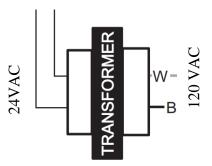
Figure 6-8 Transformer Wiring
