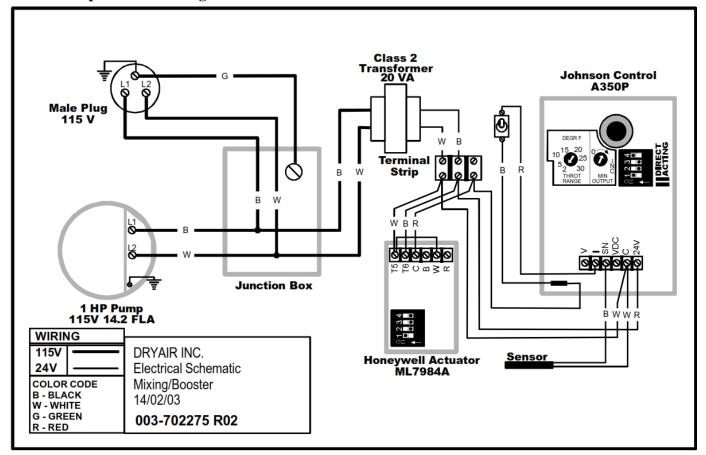
Figure 8-11 Model Pump Booster Mixing Valve
