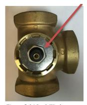
Figure 5-14 Lock Washer (Locked)
