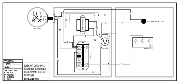
Figure 8-13 Model Humidistat Fan Coil Control
