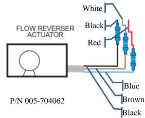
Figure 6-1 Flow Reverser Actuator Wiring
