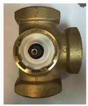
Figure 5-16 Valve Stem in Place
