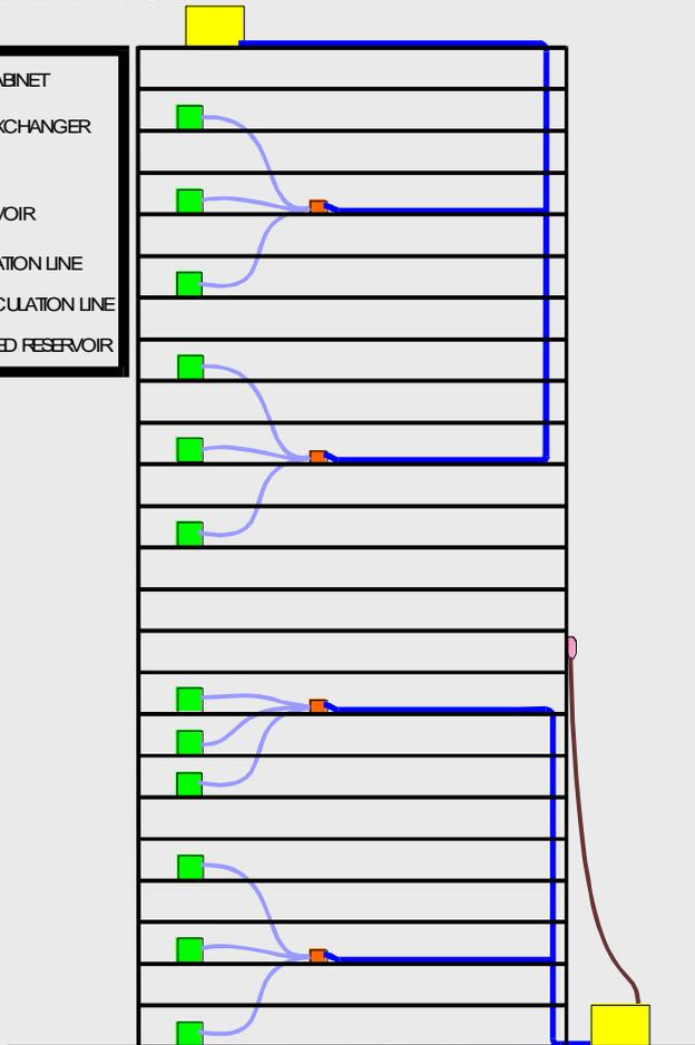
Example of a high rise layout. This layout has 2 DryAir units, one on the ground level to supply heat to the lower floors. One on the roof to supply heat to the upper floors.
