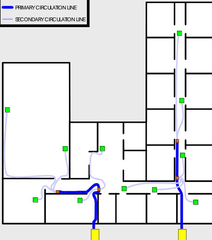
Example of a larger structure layout. This layout has 2 DryAir units, both on the ground level to supply heat to different areas of the building.
