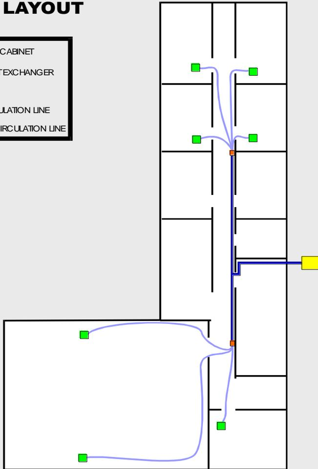
Example of a school layout. This layout has a DryAir unit, a two way primary line, and manifolds to secondary lines running to portable heat exchangers.
