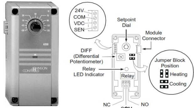
Figure 6-14 Johnson (A350A/B) Electronic Temperature Control
