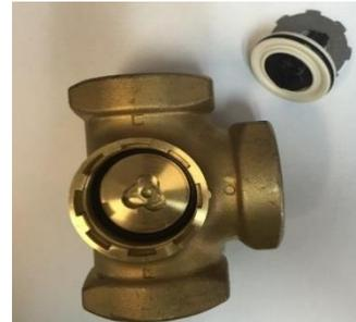
*Figure 5-17 Valve Stem Removed*
