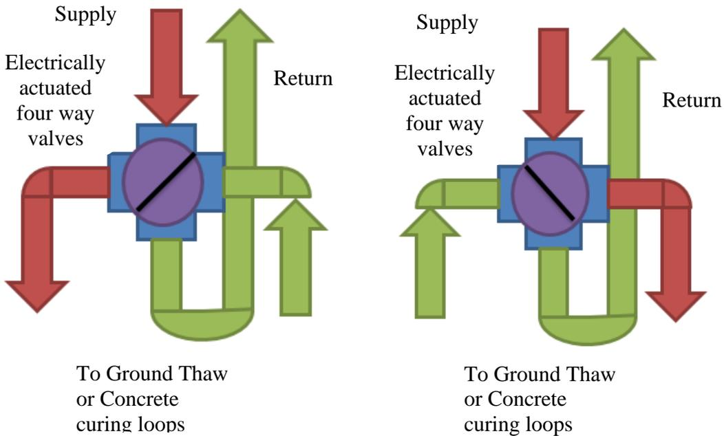
Figure 5-10 Flow Reverser Schematic
