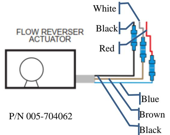
Figure 6-1 Flow Reverser Actuator Wiring
