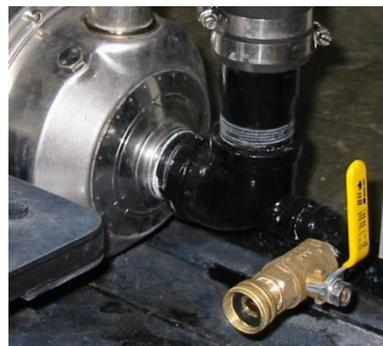
*Figure 5-5 Drain Valve*
