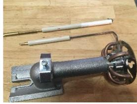
Figure 9-7 Electrodes Removed
