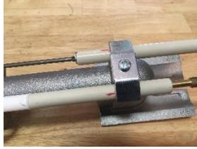
Figure 9-6 Mark Electrode Positions
