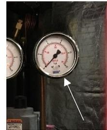
Figure 4-11 Gas manifold pressure gauge
