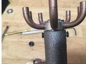
Figure 9-10 Distributor Head Screws
