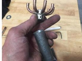
Figure 9-11 Distributor Head Removed
