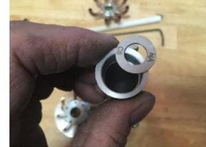
Figure 9-13 Diaphragm (Orifice)
