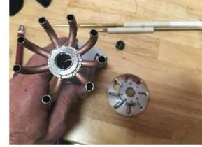
Figure 9-9 Diffuser Removed
