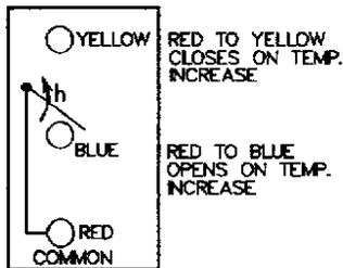
**Fig. 4 – Terminal arrangement of SPDT models.**
