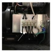
Figure 8-1 Burner Electrical Connections
