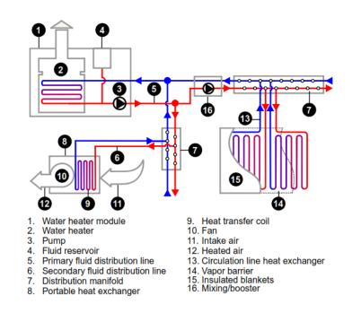
Figure 3-7How the System Works
