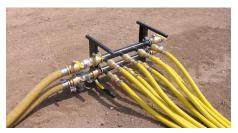
Figure 3-3Remote Manifold
