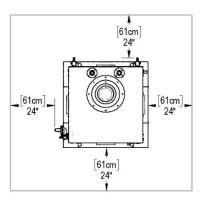
Figure 4-1Top View Clearances
