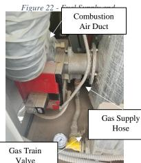
Figure 23 - Propane Gas/Natural Gas Burner Connections
