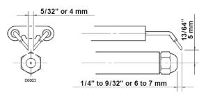
Figure 35 - Ignition Electrode Setting
