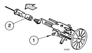
Figure 34 - Burner Nozzle
