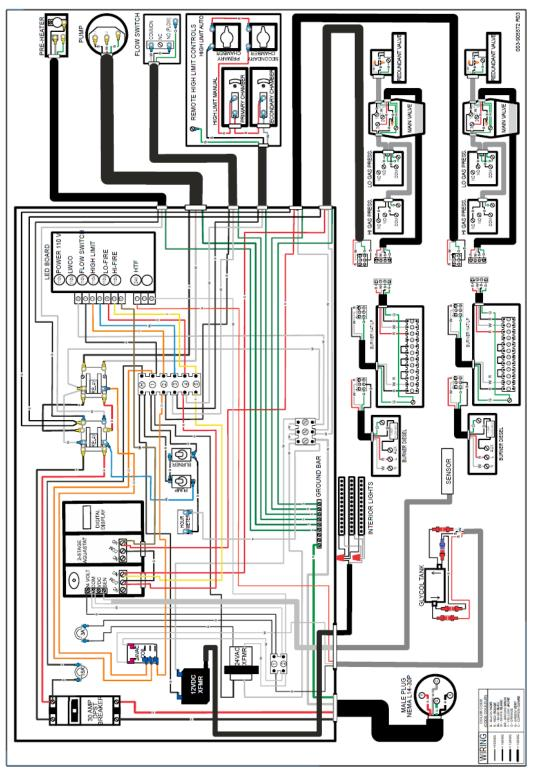
Figure 44 – 2100-DG-1800 CHU Electrical Schematic
