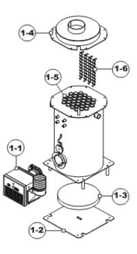
Figure 41 - Heat Exchanger Breakdown
