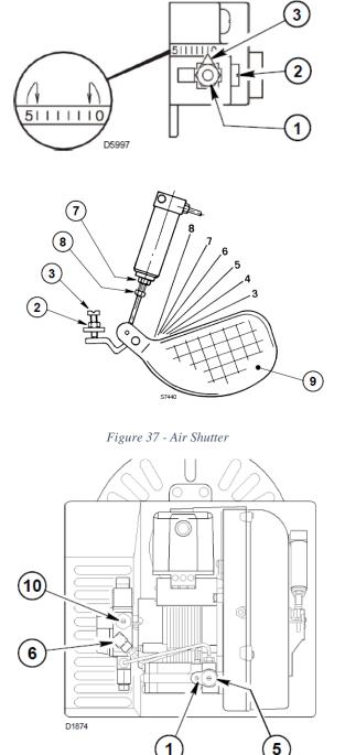
Figure 38 - Fuel Pressure Adjustment
