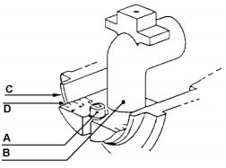
Figure 26 - Combustion Head Adjustment
