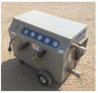
Figure 7 - Plate Heat Exchanger Unit
