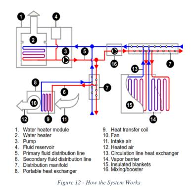
is specially designed for optimum heat transfer, without adding any moisture or combustion by-products to the air.
