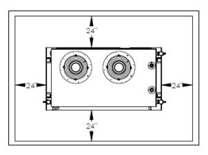
Figure 13 - Water Heater Module - Top View
