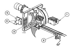
Figure 33 - Removing Burner Drawer Assembly
