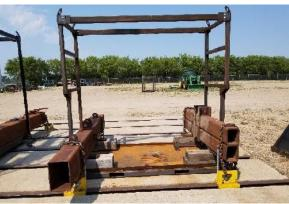
**Figure 1.** 2100x2 system base frame and installed lifting frame assembly secured to test bed.
