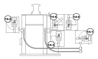
Figure 30 - Circulation Valve Positions
